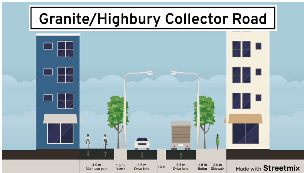
Figure 7: Granite/Highbury Collector Road cross section
